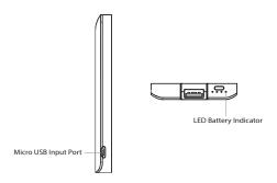
While charging, the LED battery indicator will illuminate. When battery is fully charged, the power indicator will display four solid blue lights. When fully charged, disconnect the USB to Micro USB Cable.
